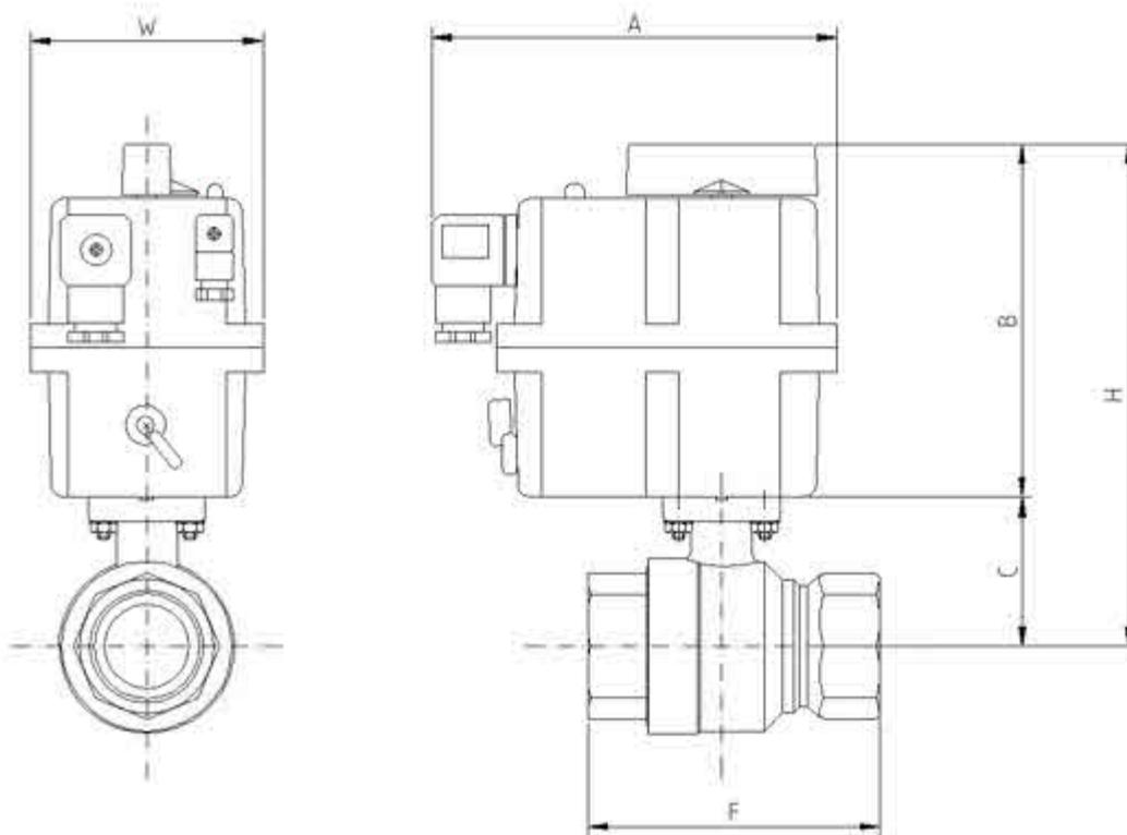
Dimensions remain unchanged for all versions (on-off, failsafe & modulating)
