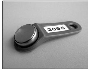
ELECTRONIC KEYS are used by pressing them to the KEY READER located on the MC's front panel.
