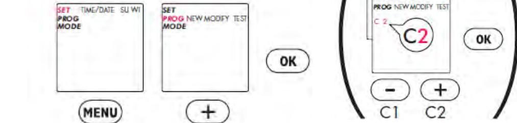
Programming: One program = switch-on time +switch-off time +switch-on and switch-off days. Programs with predefined switch-on / switch-off days. • DAY 1-7 (MO-SU) • DAY 1-5 (MO-FR) • DAY 6-7 (SA & SU). Programs for each channel are interlinked with OR logic.
