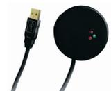
If you are using a hardwire connection then this is your RS485 port adapter using the interface shown opposite. Select the appropriate port type and number from the top dropdown list.
