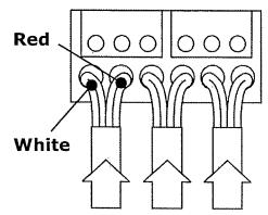
You will notice that in the probe cable there are two wires, one red and one white. The red wire should be connected to the Z(x) terminal and the white wire to the corresponding OV terminal. The colour is actually irrelevant but it is suggested for simplicity all wires to the 'OV' connections are kept the same. For Zone set-up see page 10.
