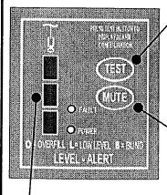
To test the alarm press and hold the 'test' button, whilst the button is pressed all the configured zones, fault, strobe and sounder will activate. If no zones are active all lights and the sounder will stop when the button is released.
