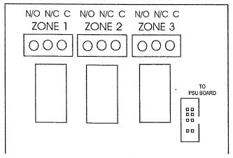
The relay outputs are optional and can be added to the unit at anytime. They allow switching to external equipment when either the High, Bund or Low alert is triggered. For example,
