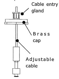
The position of the float can be adjusted to the required height by loosening the cable entry gland on the brass cap.
